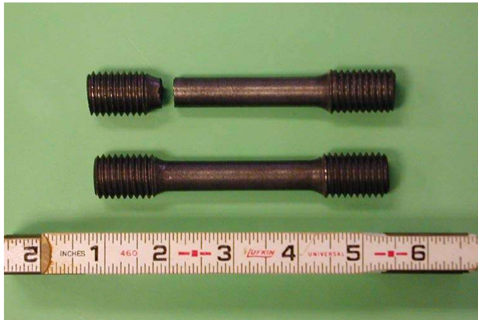
Figure 6.4.10 Brittle Fracture of Cast Iron Specimen
