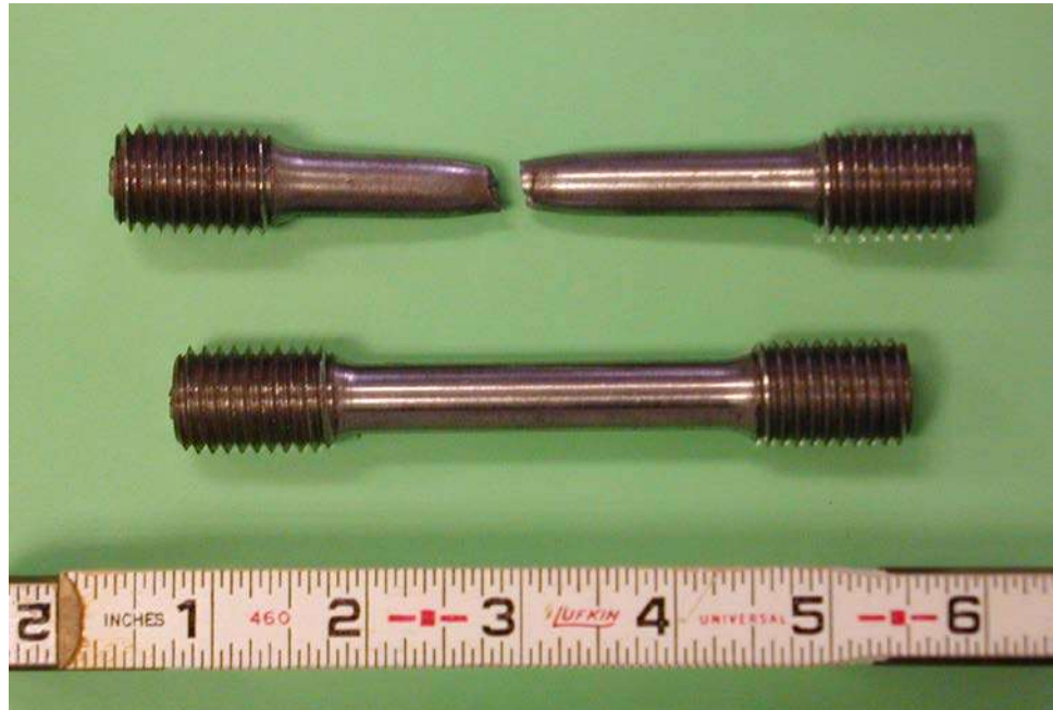
Figure 6.4.11 Ductile Fracture of Cold Rolled Steel Specimen
